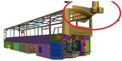
Figure 6: Designed virtual camera in the digital twin
