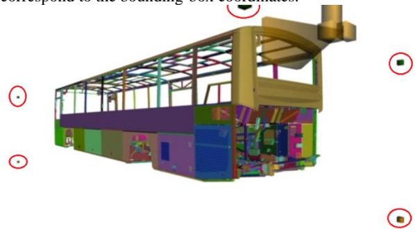
Figure 7: Bounding-box coordinates of the vehicle
