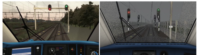
Fig. 7. Virtual environment which simulates a scenario under a) sunny meteorological conditions and b) rainy and foggy journey's meteorological conditions.
